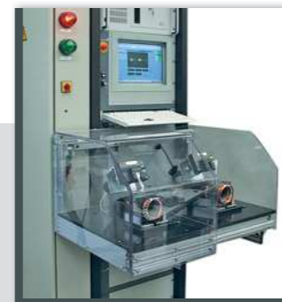
Dual station with MTC3 in 19"-cabinet
