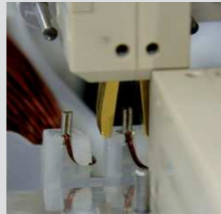
Contacting of contact pins with Kelvin clamps
