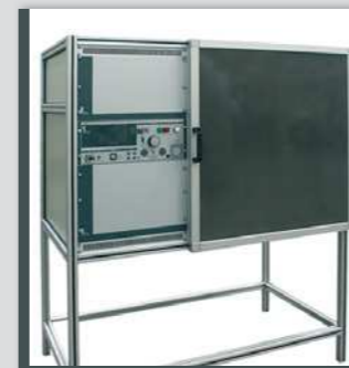
High-voltage test station up to 40KV
