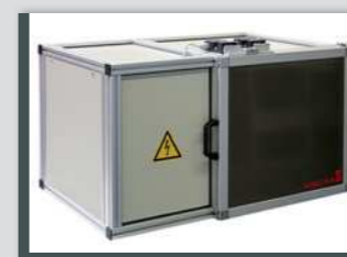
Test cage for material testing up to 40KV
