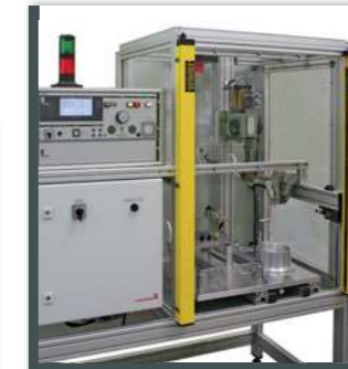
Test table with light curtain
