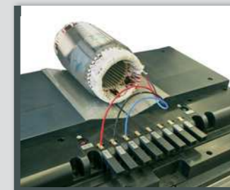
Kelvin contacting device in a test cover with prism
