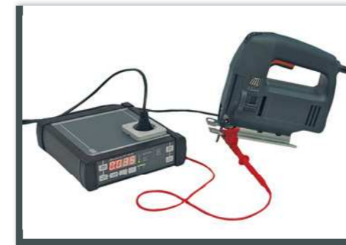
Testing PE and insulation resistance
