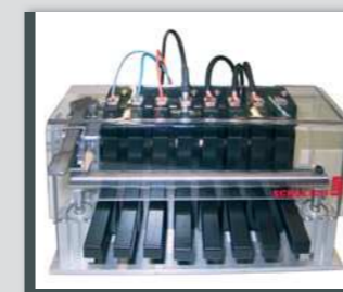
Block with Kelvin clamps with automatic release
