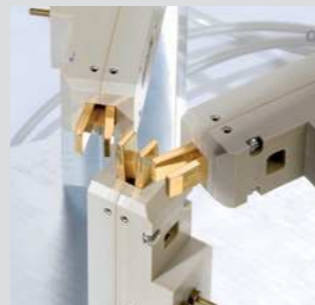
Contacting of contact pins with Kelvin clamps
