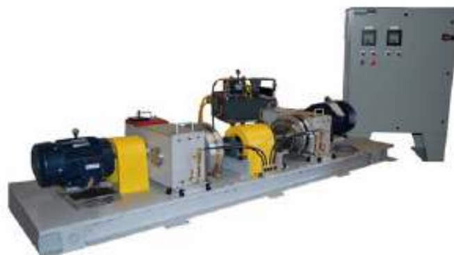
Turbine Blade Crack Research Test Rig This test machine is specifically designed to simulate turbine blade crack and includes advance telemetry Instrumentation.
