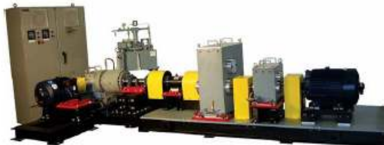
Drive-train/Gearbox Diagnostics/Prognostics Test Rig Designed to perform prognostics tests on special gearbox and bearings for petroleum industry.
